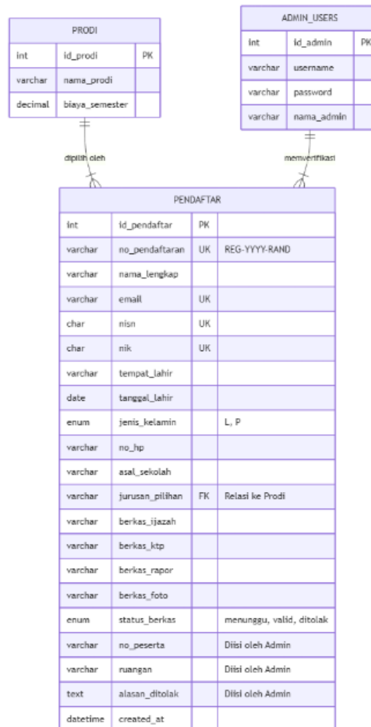
Gambar 3. Entity Relationship Diagram (ERD)
