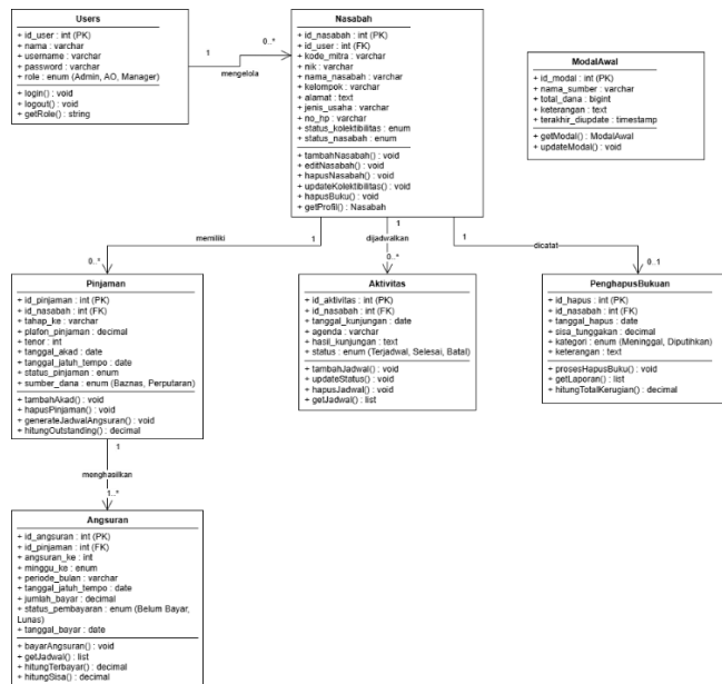
Gambar 8. Class Diagram Arsitektur Basis Data Sistem CRM
