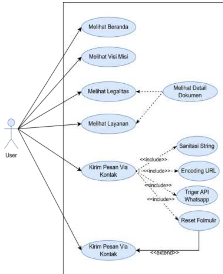
Gambar 2.1 Use Case Diagram Sistem Usulan
